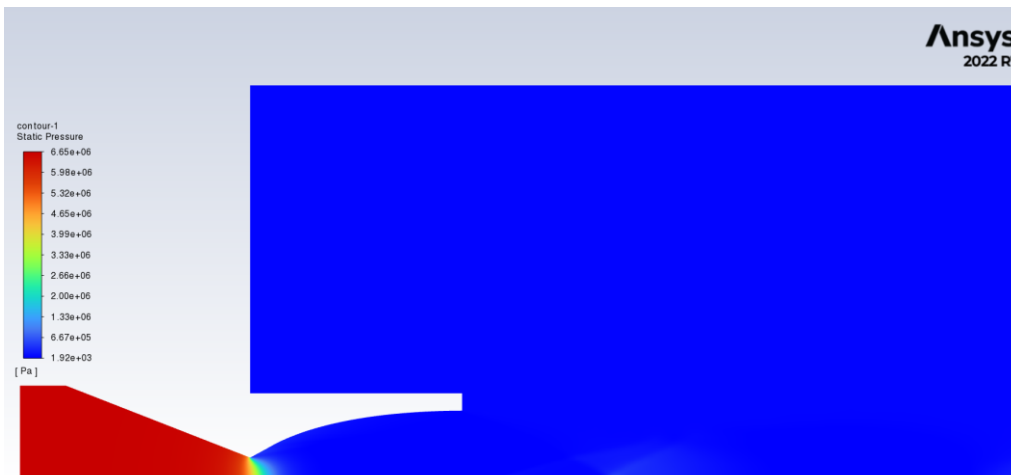
Figure 4.25 – 10% geometry decrease static pressure contour.
