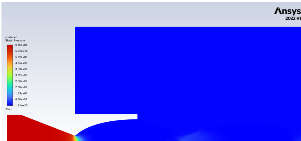
Figure 4.34 – 2.5% geometry increase static pressure contour.
