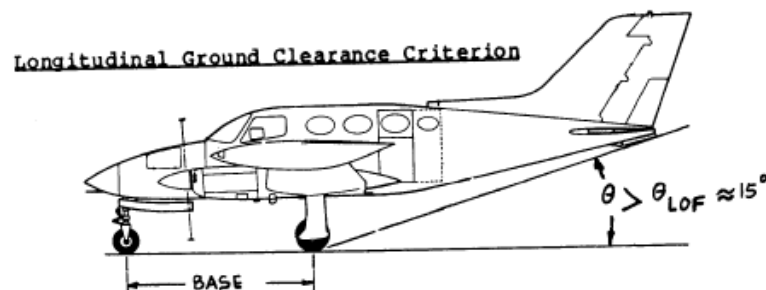
Figure 158: Longitudinal ground clearance criterion for tricycle gear
