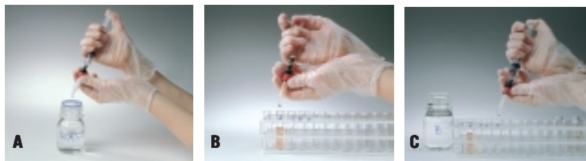
Fig. 3. Using GSTrap with a syringe. A Prepare buffers and sample. Remove the column's top cap and twist off the end. B Load the sample and begin collecting fractions. C Elute and continue collecting fractions.
