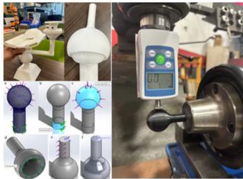
Figure 2. Arm support design: fully 3D-printed assembly featuring a ball-and-socket joint (upper left); mesh models of the ball joint and socket joint (lower left); and force testing of the printed component (right).
