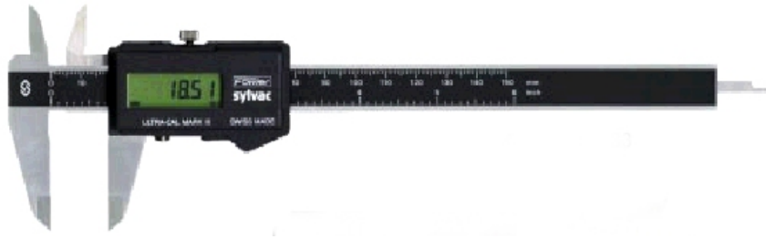
Figure 3 Electronic caliper. This model uses a capacitive sensing approach to measure the distance between the two jaws. It also can be interfaced to a personal computer using an RS-232 cable, so that measurements can be recorded automatically.
