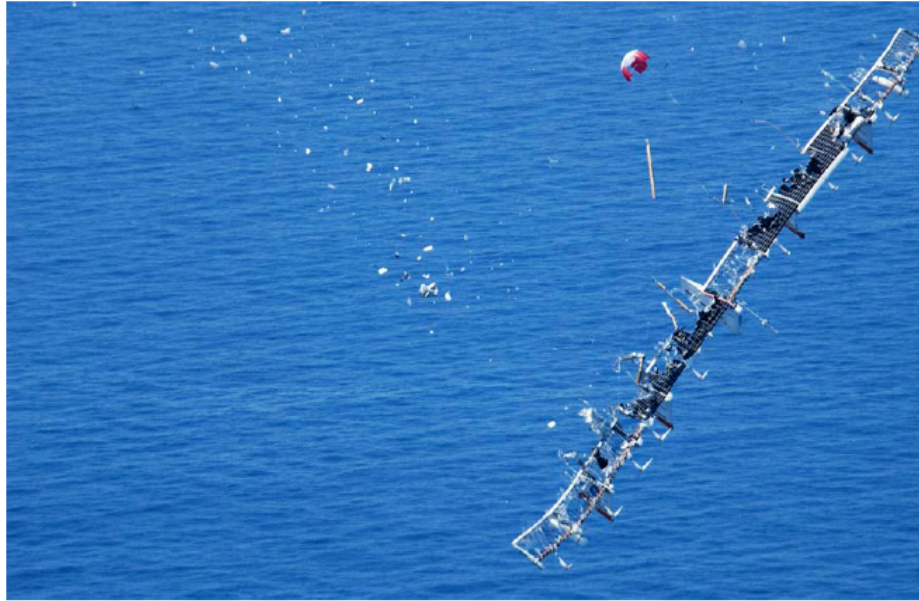
Figure 9: Helios HP03 Complete Structural Failure [3]
