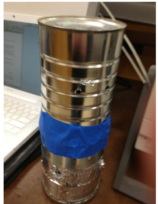
Figure 6 Coffee can waveguide filter 4" in diameter
