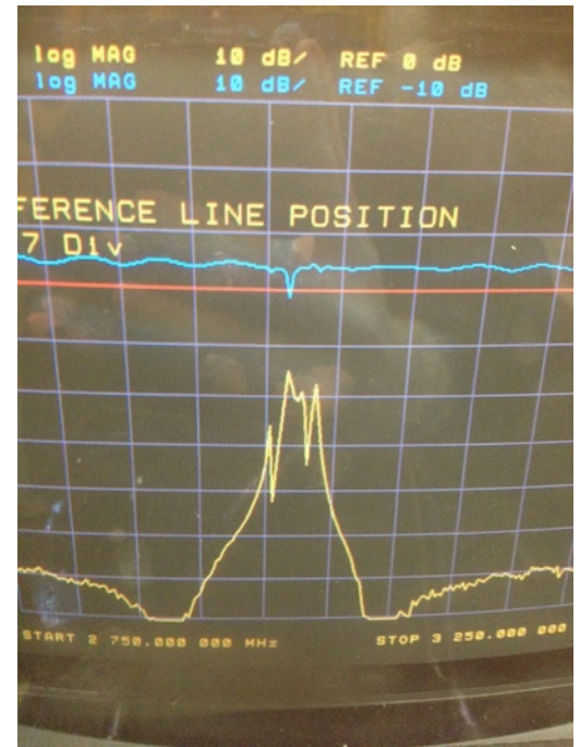
Figure 7 Measurements from the Network Analyzer showing S_{11} and S_{21} that shows the four peaks from the four elements
