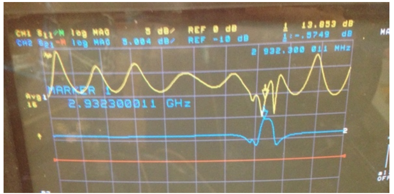
Figure 9 After tuning and calibration of the network analyzer, three peaks have been combined
