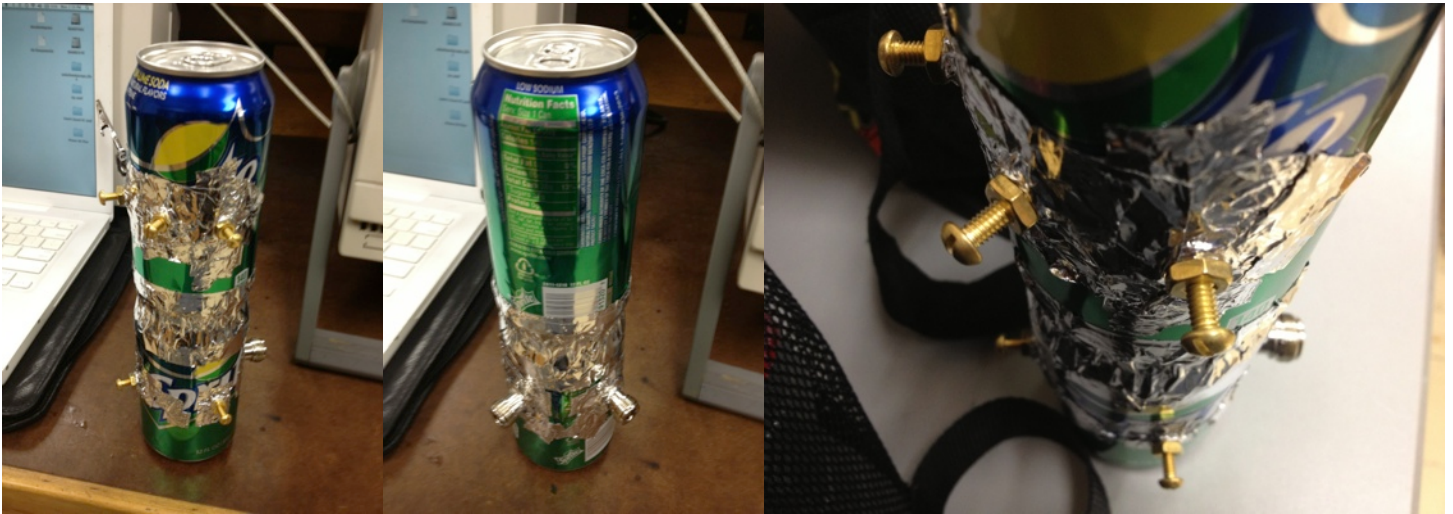
Figure 5 Soda can canonical waveguide filter 2.5" diameter
