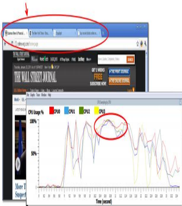
Figure 5. CPU usage percentage vs Time of one browser with multiple tabs in quad core.
