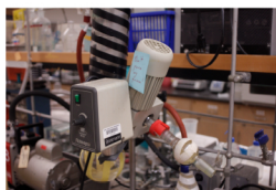
Image 4: Rotary Evaporator, used to remove methanol from the sample
