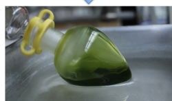
Image 5: Spinning round bottom flask; evaporation in progress
