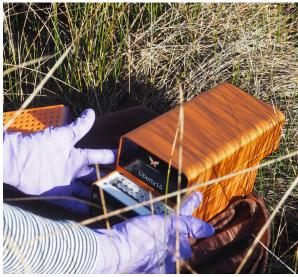
$A BOVE: Handheld\,qPCR\,instrument\,that\,can\,detect\,DNA\,from\,target\,HAB\,species.$
